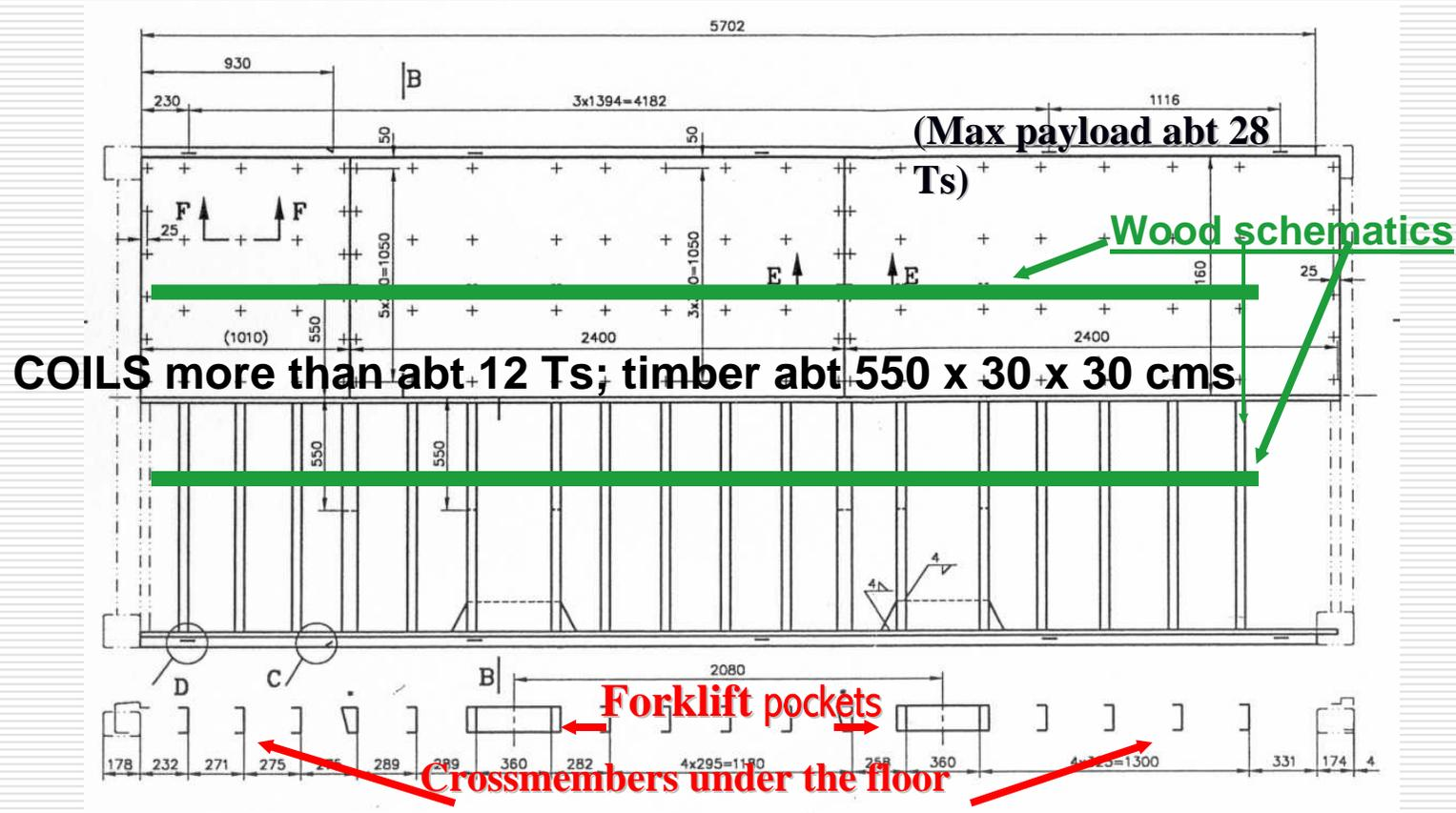
Always min. 2x layers in the width and never any coil touching the floor.
