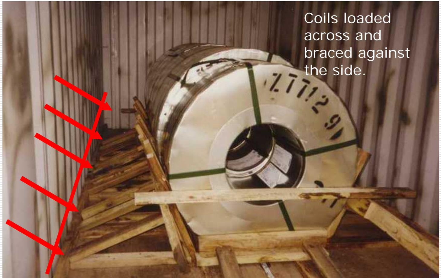
Coils loaded across and braced against the side.
